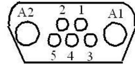
**Output Connector Pin Assignment**
